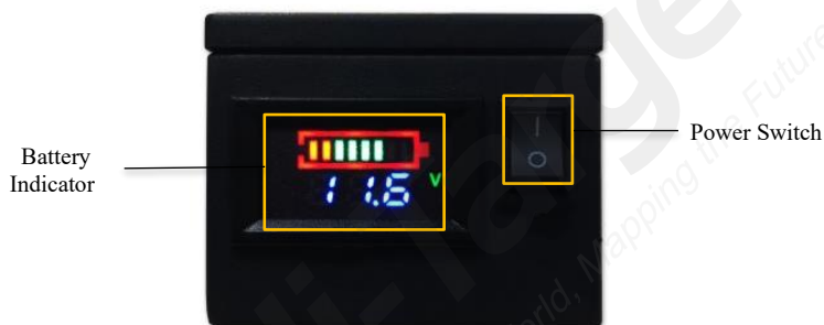
Figure 1-6 Working state of the battery
